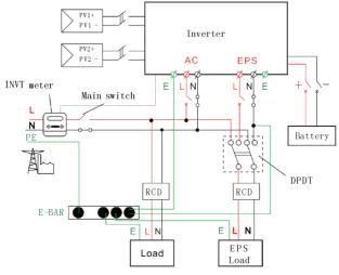
I Version applies to the wiring rules that requires Neutral line of alternative supply must NOT be isolated or switched (applies to wiring rules AS/NZS\_3000:2012 for Australia and New Zealand).
