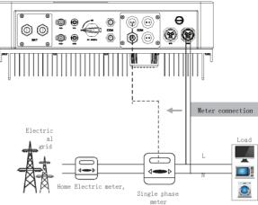
Meter PIN Definition Communication interface bewteen inverter and meter is RS485 with a RJ45 connector.
