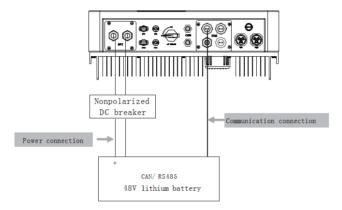
Note: When working with Pylontech batteries, It is recommended the number of battery module (H48050-15S) is 2-7 and the number of battery manager system (SC0500A-100S) is 1.
