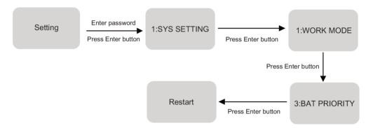
Note: When choosing battery priority mode, the corresponding charging current should be opted for according to the battery type. The system default current is 25A.
