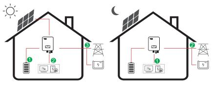
**Energy flow:**  $PV \rightarrow Battery \rightarrow Load \rightarrow Grid$
