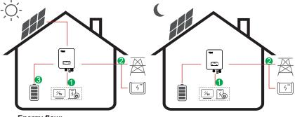
Energy flow:  $PV \rightarrow Load \rightarrow Grid \rightarrow Battery$
