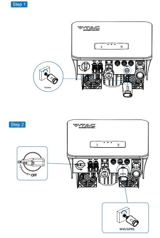
Turn on the DC switch and AC circuit breaker, and wait until the LED indicator on the monitoring module flashes, indicating that the monitoring module is successfully connected.
